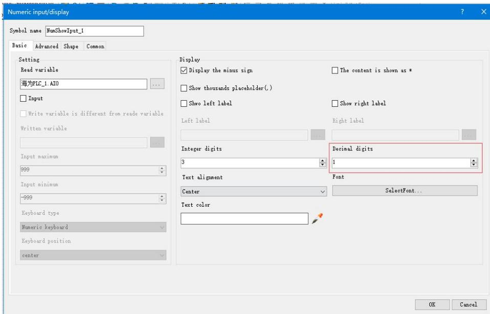
So that when the PLC read AI0 value, AI0=123, that is the actual value of 12.3°C, there is no need to have data processing in PLC and configuration, only set the 1 decimal places on the numerical display primitive, then it will be automatically reduced by 10 times, displaying value of 12.3, that is the actual value of 12.3°C.
